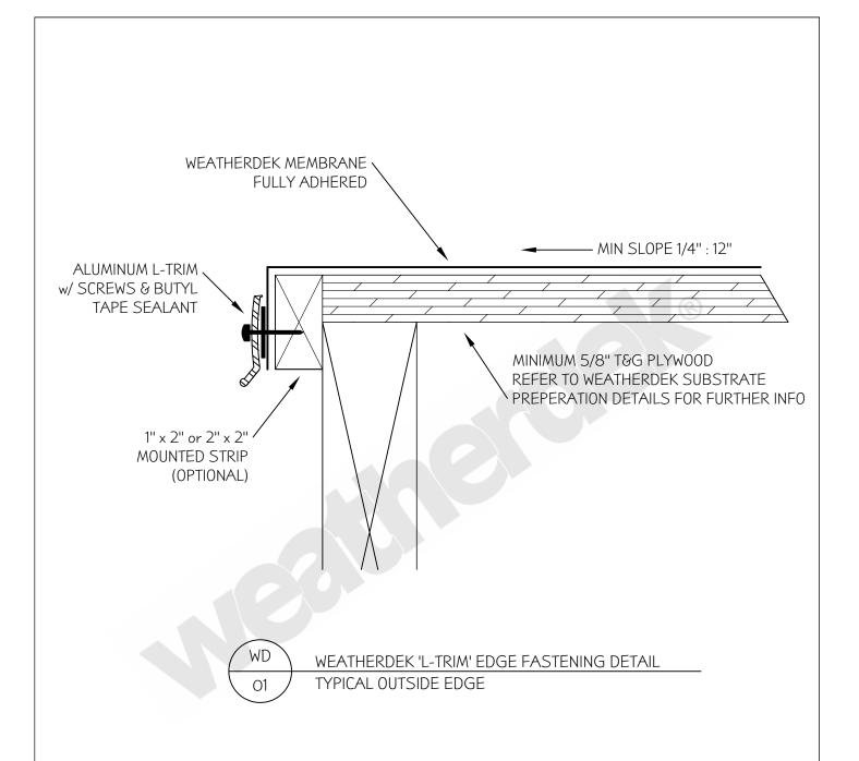
NOTE: AS A SUPPLIER OF MATERIALS ONLY ADS WEATHERDEK DOES NOT ASSUME RESPONSIBILITY FOR ERRORS IN DESIGN OR SITE CONDITIONS. SUITABILITY OF ALL DETAILS SHOULD BE CONFIRMED BY THE ARCHITECT, CONTRACTOR OR OWNERS REPRESENTATIVE.
